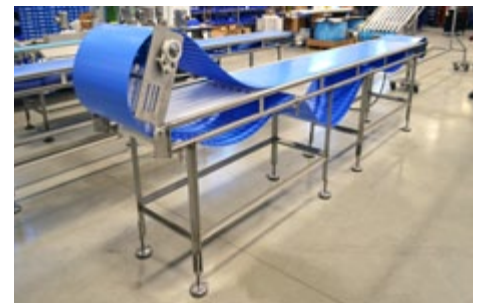
Idler end flips up to release belt tension for easy access to remove, clean and sanitize internal components.
