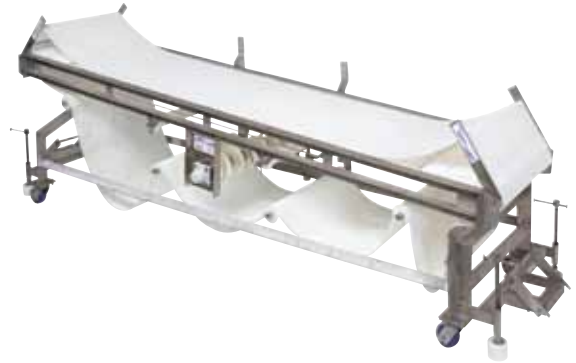
Flip-up ends to release belt tension
